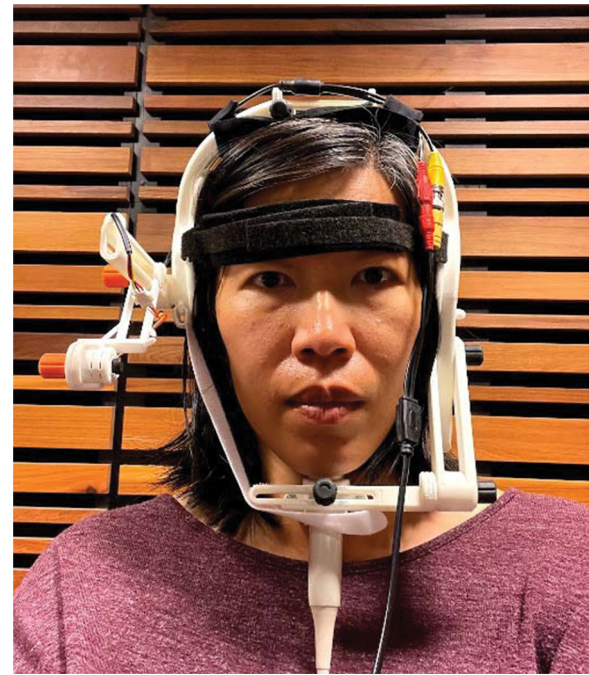
FIGURE 1 UltraFit headset holds the convex 20 mm radius ultrasound transducer in a midsagittal position while a side-mounted camera monitors the bolus approaching the mouth [Colour figure can be viewed at wileyonlinelibrary.com ]
